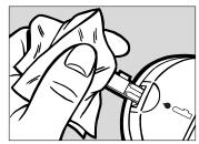
4 If you want to store the test result, remove the Test Strip from the Meter as shown. The Meter turns off automatically and the test result is now stored in the memory. You may wish to use a tissue or the foil wrapper from the strip to remove the used strip.
